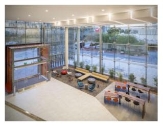
The glass and systems: High-performance, low-emissivity coated glass allows expansive natural light to move through the building while managing the Las Vegas desert sun's accompanying heat, bringing value to the building's overall operations by helping the HVAC system run efficiently.
